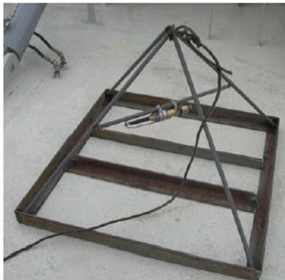
Figure 5 Hydrophone attached to an example of a seabed cage
